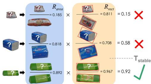
Figure 3. Samples of pose selection. The stability factor  $R_{stable}$  is the product of  $R_{area}$  and  $R_{rect}$ . The unstable poses with stability factor less than  $T_{stable}$  are removed.
