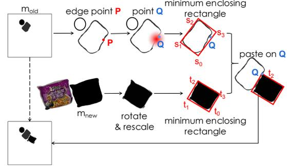
Figure 4. Instance placement. We randomly choose an edge point  $P$  from  $m_{old}$  and sample a surrounding point  $Q$ . The nearest edge of the MER of  $m_{old}^i$  of  $P$  to  $Q$  is  $(s_0, s_3)$ . We compute MER for the new instance  $m_{new}$  after rotation and re-scaling and randomly choose  $t_2$  from  $\{t_1, t_2\}$  to paste on  $Q$ .
