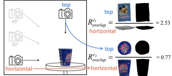
Figure 5. The overlap factor for each category is the ratio of two areas: the minimum area of mask from the top view and the maximum area of mask from the horizontal view.
