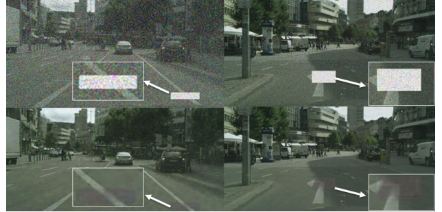
Figure 4: Results on CS Dataset: The autoencoder manages to remove the noise and utilize the temporal aspect to restore the missing line and arrow on the road.
