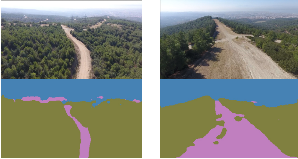
Figure 2: Example of semantic segmentation performed on drone-captured RGB video data.
