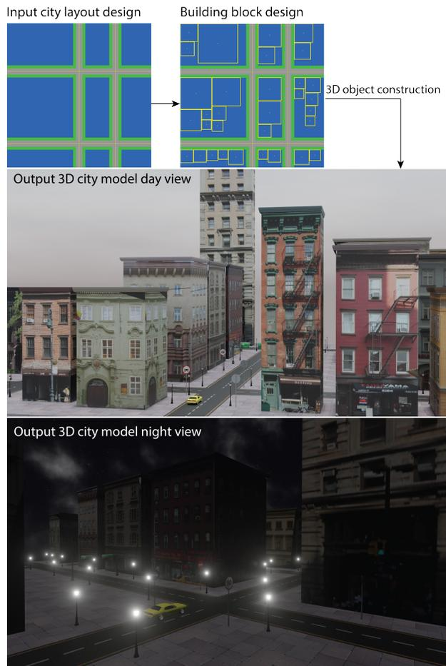
Figure 1: In this paper we introduce a pipeline that takes a simple 2D layout image as input and outputs a virtual 3D city model according to the specified design. The output model consists of important city elements: building blocks, road systems and street lamps. Each building is textured with a real-world building facade. Specific objects, such as road signs, can be added to these scenes to provide additional training and evaluation data for deep learning-based detection algorithms.
