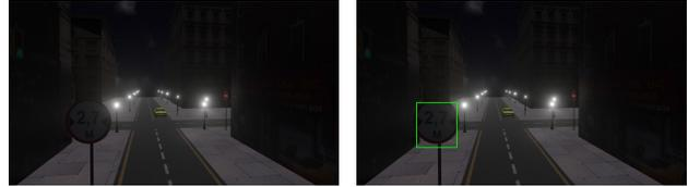
Figure 14: Prediction examples of traffic sign detector trained with different synthetic image dataset rendered from our output 3D city. Left: prediction result of the object detector trained with only daytime images and it failed to detect the road sign in a nighttime image. Right: prediction result of the object detector further fine-tuned with nighttime images and the road sign was successfully retrieved under extremely low illumination.
