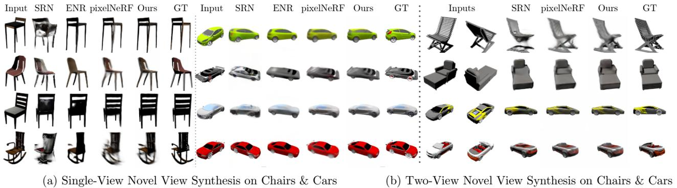
Figure 3: **Qualitative results on category-specific single chair & single car.** The model can either take (a) single view or (b) two views as input to synthesis novel views. We find similar rendering quality comparing to pixelNeRF [49] and better geometry prediction comparing to ENR [7] and SRN [35].
