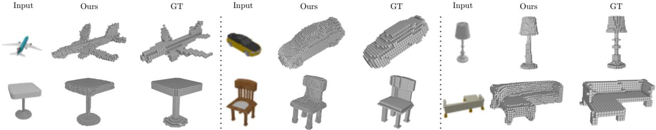
Figure 6: **Qualitative results for 3D geometry reconstruction.** We visualize the predicted  $\alpha$  volume with its raw resolution  $64^3$  and the ground truth volume with its raw resolution  $32^3$ . With a single-forward pass, our model can perform 3D geometry reconstruction given a single view of objects from 13 different categories. Our model trained with only 2D supervision consistently predicts meaningful and full geometry.
