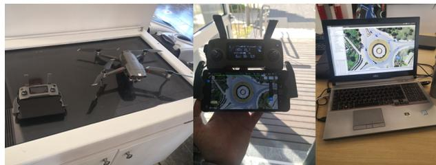
Figure 7. 1) DJI Mavic is used to capture traffic video data. 2) The video is streamed through a local network. 3) A NGIX service is running on laptop to receive video and process it in real time
