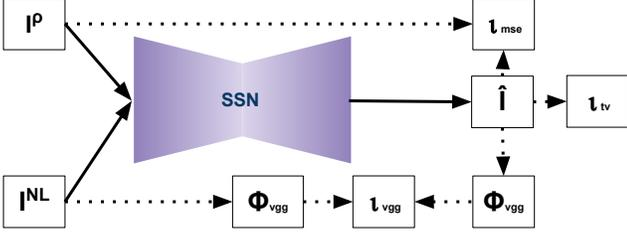
Figure 4. **Self-Supervised Network (SSN)**: We train SSN on a combination of three losses that are  $l_{mse}$ ,  $l_{tv}$ , and  $l_{vgg}$ . We use  $l_{mse}$  to get the average content of priors  $I^\rho$ .  $l_{tv}$  is then used to minimize the small rainy streaks. We use  $l_{vgg}$  to improve the high-frequency information in the output image  $\hat{I}$ . The dotted line represents the flow of input to a loss function, and the solid line shows the flow of input and output to the SSN.
