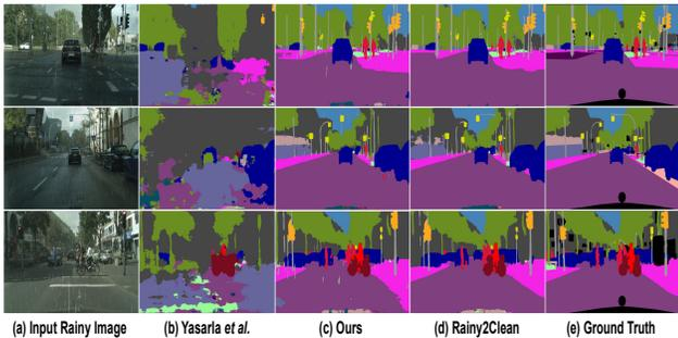
Figure 10. **Semantic Segmentation Results:** Visual segmentation results obtained by ERFNet on images derained from different methods.
