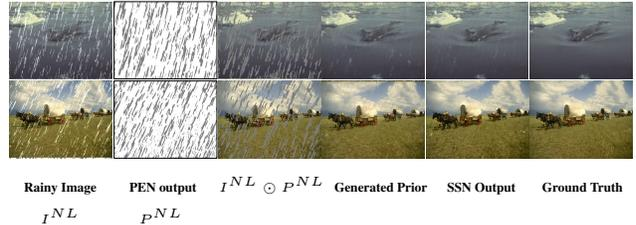
Figure 3. **Visualization of output at various stages:** Left to Right: col. 1: input rainy image, col. 2: PEN output, col. 3: masking of rain by taking the dot product between rainy image and PEN output, col. 4: output obtained from image inpainting, col. 5: refined output from Self-Supervised Network.
