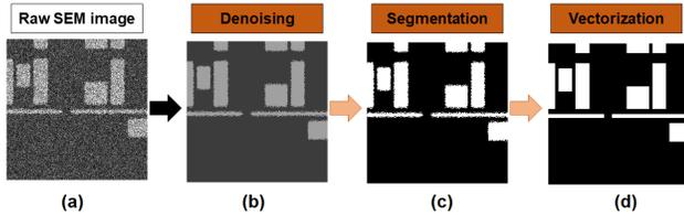
Figure 2. The image processing pipeline for hardware assurance
