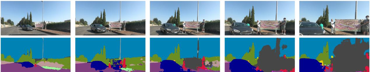
Figure 12: Illustration of the real-world adversarial patch effect on sequential frames processed by the ICNet model.
