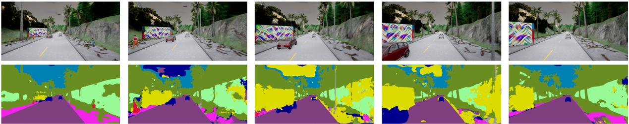
Figure 11: Illustration of the adversarial patch effect on CARLA simulator showing sequential frames of scene 1 processed by the BiSeNet model
