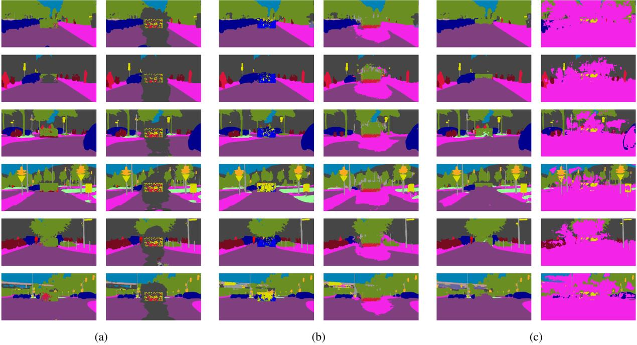
Figure 3: Semantic segmentations obtained from DDRNet (a), ICNet (b), PSPNet (c). For each block, the first column represents SS obtained from images patched with random patches ( $200 \times 400$ ), while the second column refers to images patched with patches crafted with EOT-based attack.
