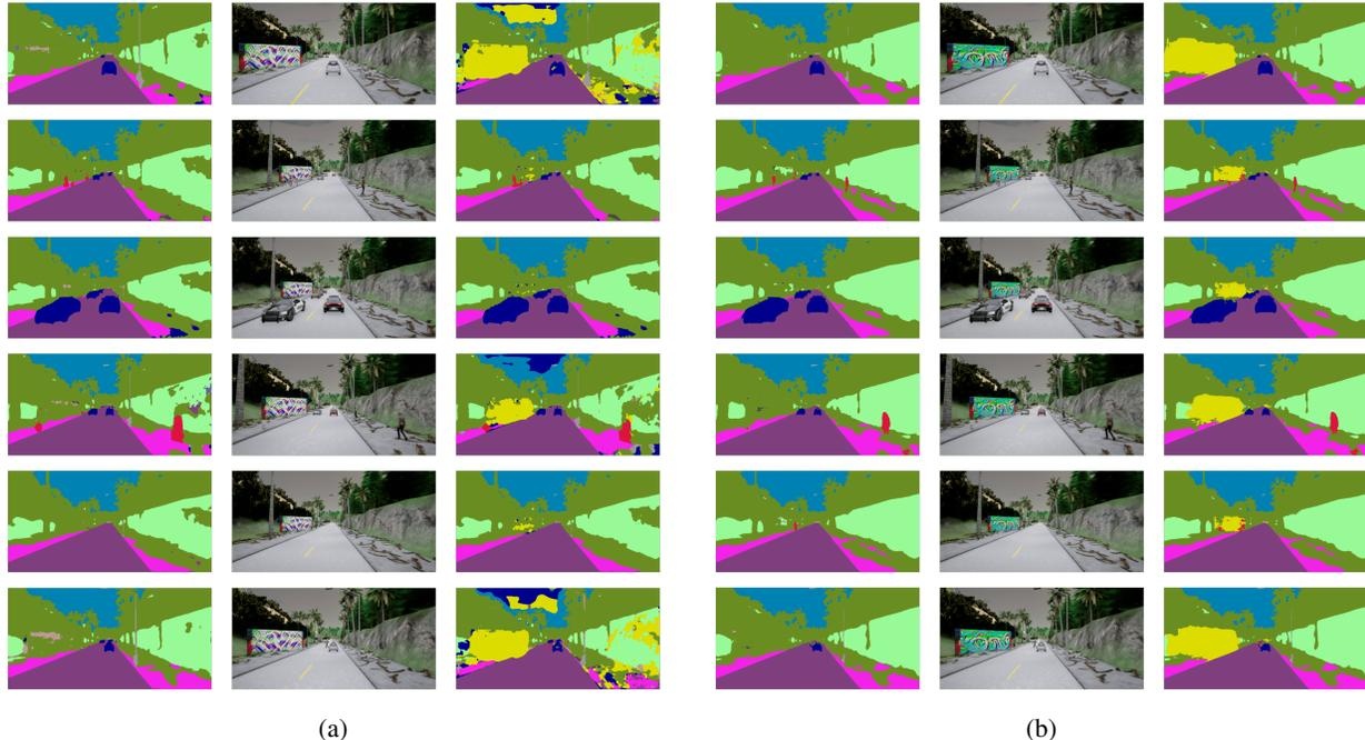
Figure 7: Semantic segmentations obtained from BiSeNet (a) and ICNet (b) on CARLA Scene-1. For each block, the first column is the SS obtained from images patched with random patches, the second represents the patched image with the patch optimized with the scene-specific attack, and finally, the third column is its predicted SS.
