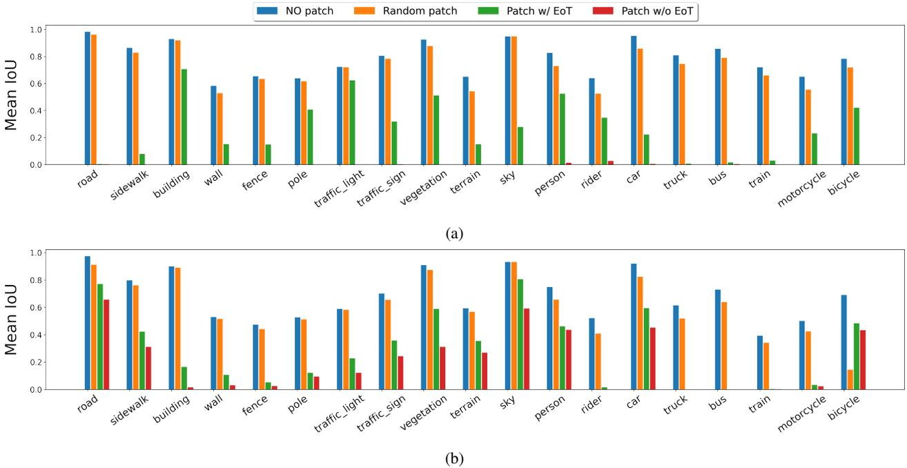
Figure 4: Per-class mIoU comparison on Cityscapes. Each bar shows the mIoU associated to a certain class, computed on the validation set. The results provide a comparison between 4 different cases: no patch applied into the images (original dataset), random patches, EOT-based and no-EOT-based patches. The reference networks were PSPNet (a) and BiSeNet (b).
