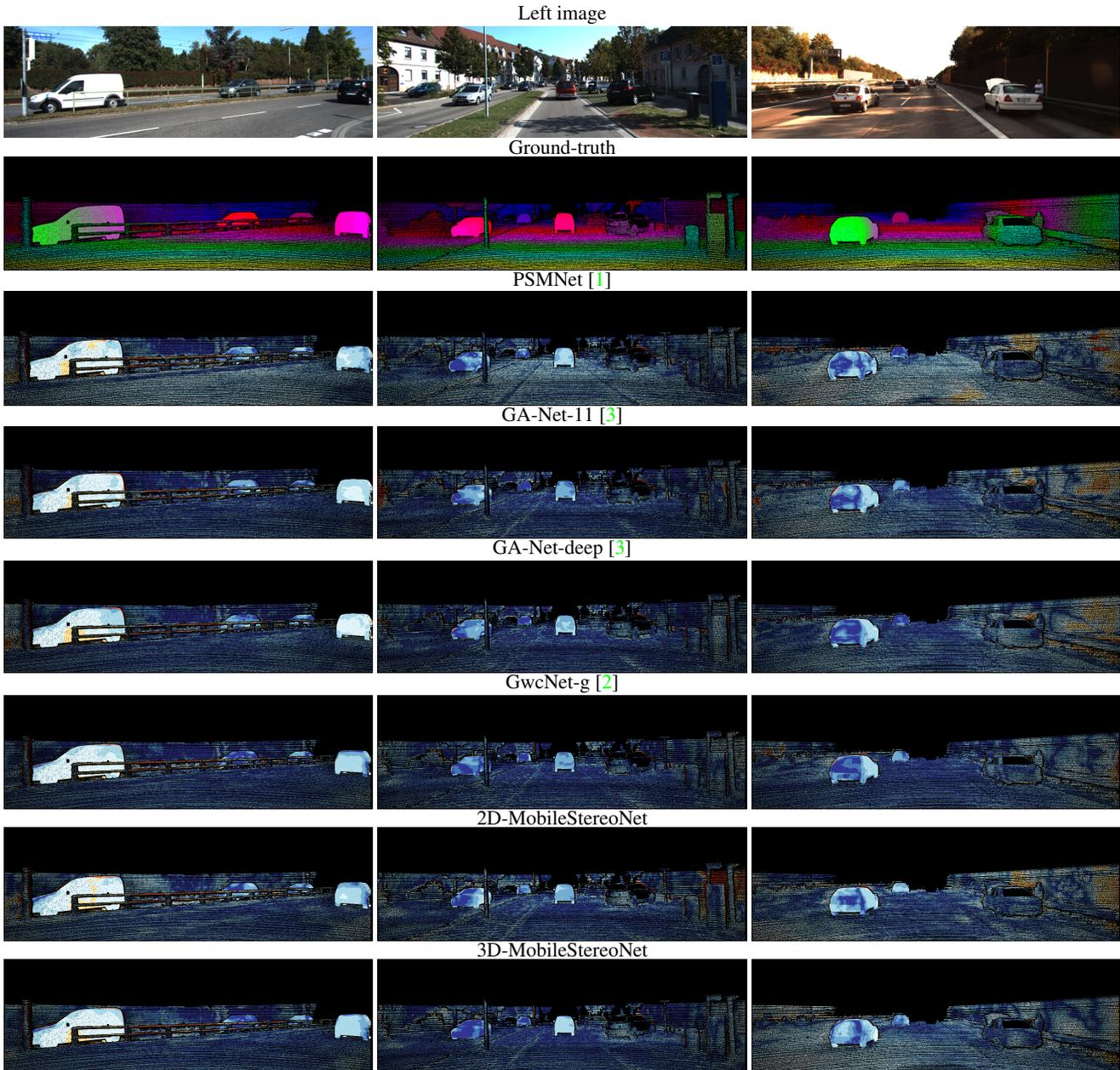
Figure 3: Qualitative performance on KITTI 2015 validation set: From top to bottom, the left image, the ground-truth disparity map and the estimated disparity maps by PSMNet [1], GA-Net-11 [3], GA-Net-deep [3], GwcNet-g [2], 2D-MobileStereoNet and 3D-MobileStereoNet are illustrated. For a fair comparison, we trained all the models with a 159/40 split of KITTI 2015 training test. Warmer colors in error maps denote higher errors.
