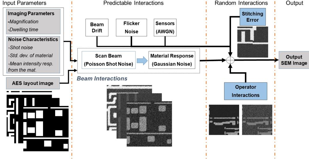
Figure 1. Workflow for generating a synthetic SEM image for the REFICS dataset.
