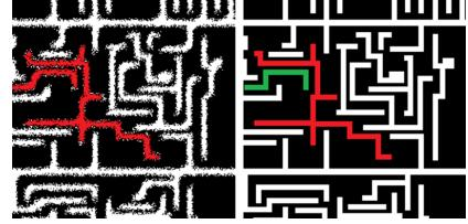
Figure 3. Imperfections introduced by the segmentation algorithms. Tiny hairline connection exists between the red components highlighted on the left leading to a false short circuit (under-segmentation). Original layout is shown on the right for comparison.
