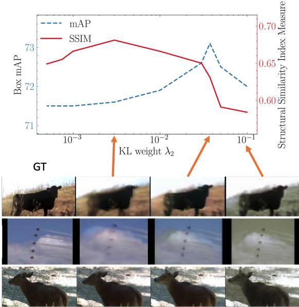
Figure 6: Effect of varying the KL loss weights on the detection and generation accuracy, showing the synthesized 10th frames corresponding to the weights and the corresponding ground truth.
