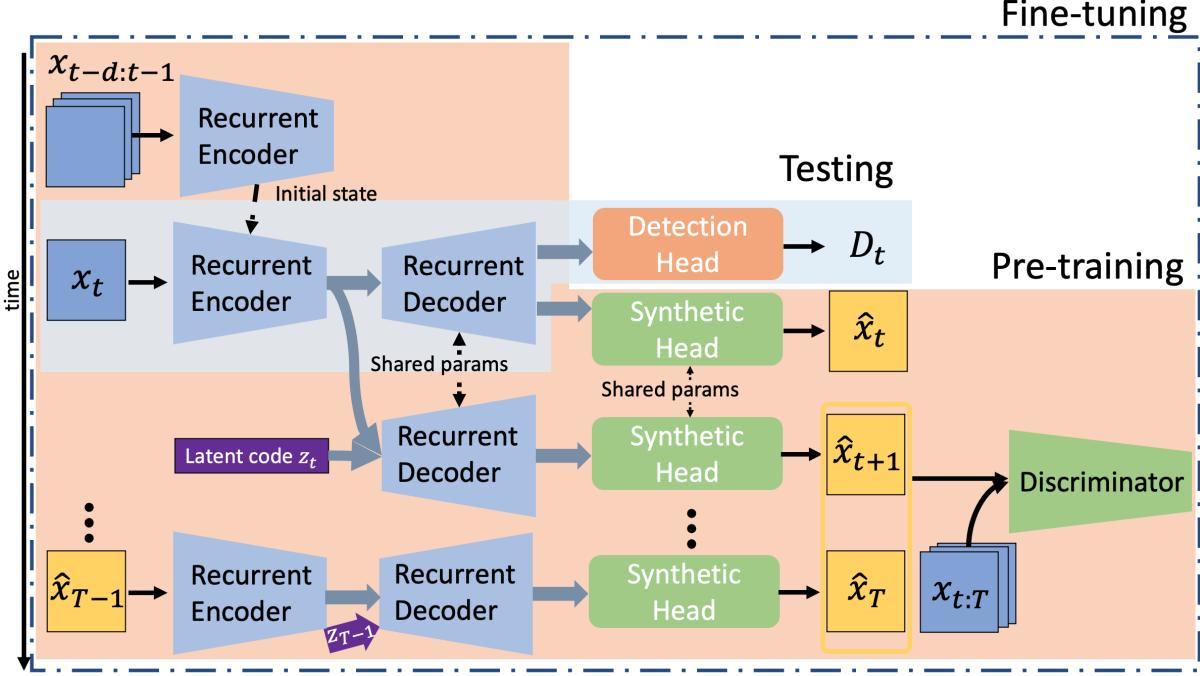
Figure 3: The architecture of the proposed model. The model is pre-trained using the components in the orange-colored area, and then fine-tuned using the whole components. The inference corresponds to blue-colored area.
