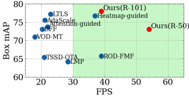
Figure 2: Accuracy-speed trade-off across various online detectors on ImageNet VID (our method is plotted in red, using ResNet backbones). Green color area represents real-time performance.
