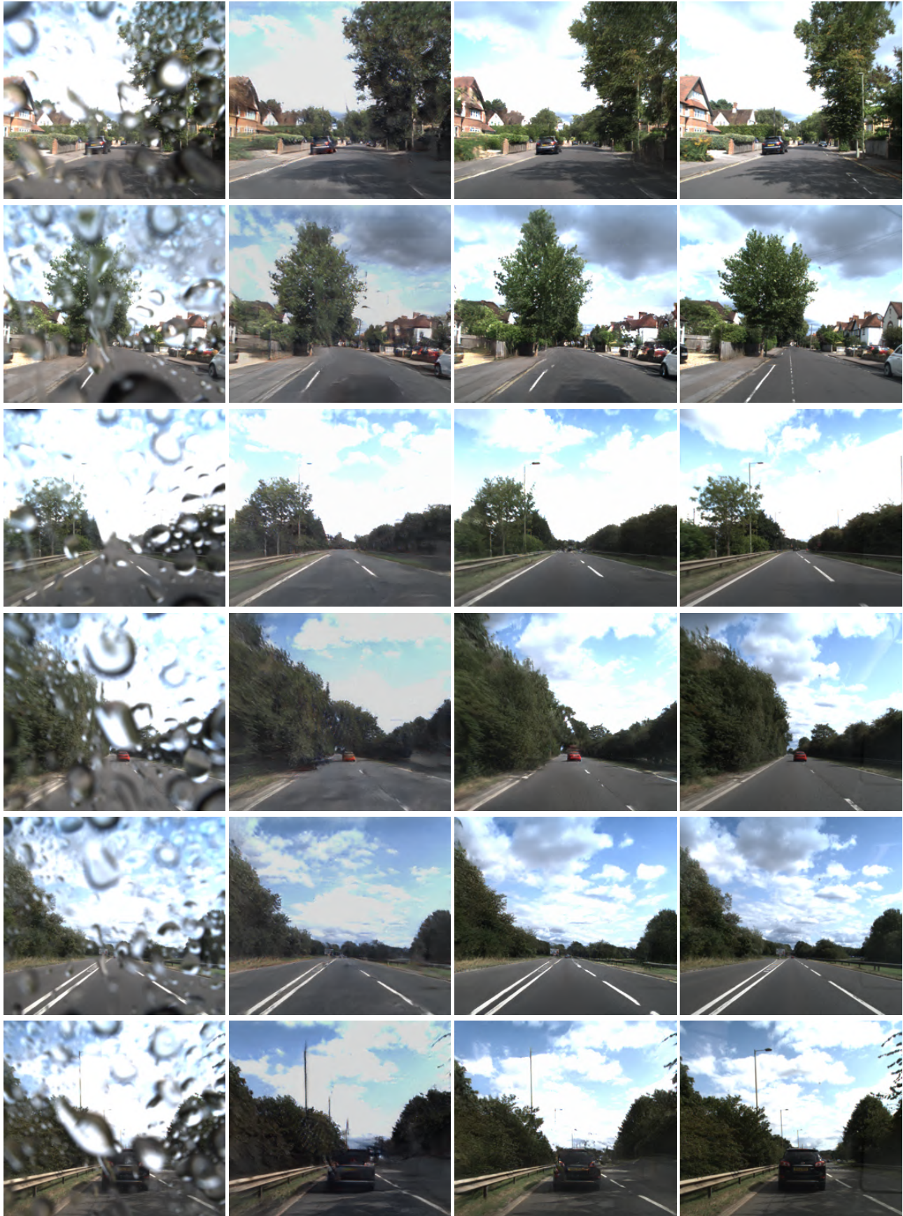
(a) Raindrop (b) CycleGAN (c) Ours (d) Groundtruth Figure 2. Visual comparison with CycleGAN[4]. From left to right: Raindrop image, CycleGAN, Ours, and Groundtruth
