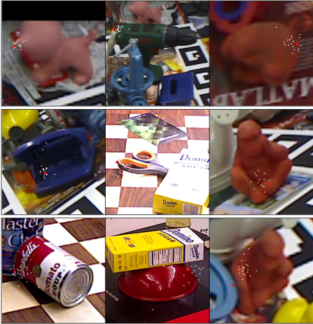
Figure 5: Deformable attention sampling locations. The red circle indicates the reference point while the white circles indicate deformed sample positions. On the last column, we show attention sampling for the same object and keypoint, with the first row having the keypoint visible whereas on the bottom two the keypoint is self or externally occluded. When the keypoint is occluded, attention learns to sample clues elsewhere on the object silhouette.
