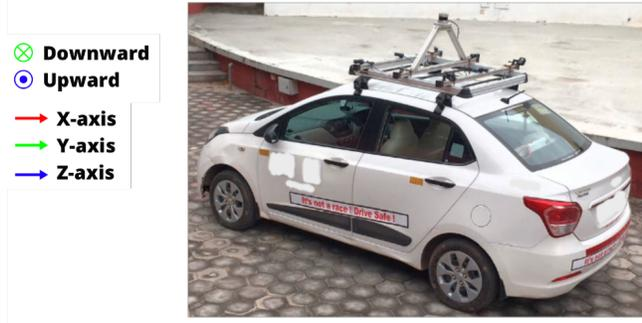
Figure 5. Figure showing (a) sensors on the vehicle (cameras, LiDAR) and their respective orientations, (b) image of the vehicle used along with the sensor rig. Please note that the real-world car image has been edited to preserve anonymity.
