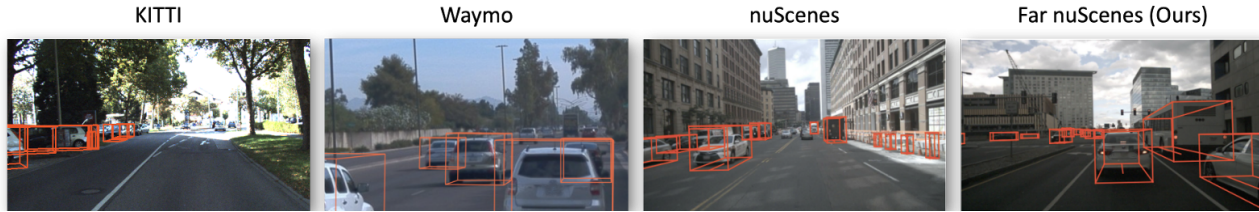
Figure 2: Ground-truth visualization for some well-established 3D detection datasets. Clearly, they (the first three columns) have significant amount of missing annotations on far-field objects (a quantitative analysis is in Fig 3). To obtain a reliable validation set, we describe an efficient verification process (in Sec 3.1) for identifying annotators that consistently produce high-quality far-field annotations. This helps us identify high-quality far-field annotations, and derive Far nuScenes (rightmost) that supports far-field detection analysis.
