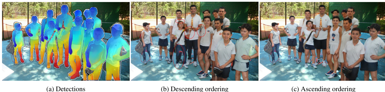
Figure 4: Anonymization results comparing our method with descending and ascending image stitching order. The ascending ordering stitches foreground objects last, which improves image quality at detection borders (e.g. marked in red).
