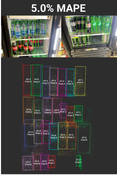
Figure 4: Example predictions from CountNet3D on real-world data. (Best viewed in color with zoom in). The PointBeam proposals, the ground truth (GT), and the predicted counts (pred) are shown. We also display the scene-level MAPE. Each beam is given a randomly generated color to highlight the beam regions. We only display the global \langle x, y, z \rangle for visualization clarity. We observe that under extreme occlusion, where both 2D and 3D object detectors are likely to fail, CountNet3D is able to accurately predict the object counts. See supplementary materials for additional image/video examples.
