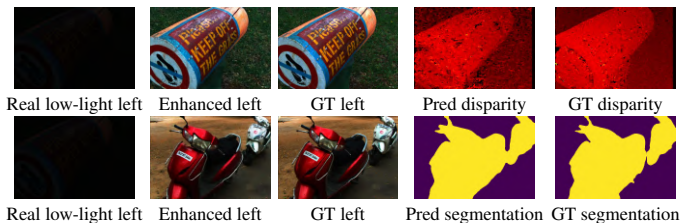
Figure 4. Qualitative results on real low-light stereo images using our network. Not only is the enhancement almost identical to the GT views but results of downstream tasks such as depth estimation and semantic segmentation on enhanced views at par with estimates obtained from GT views.
