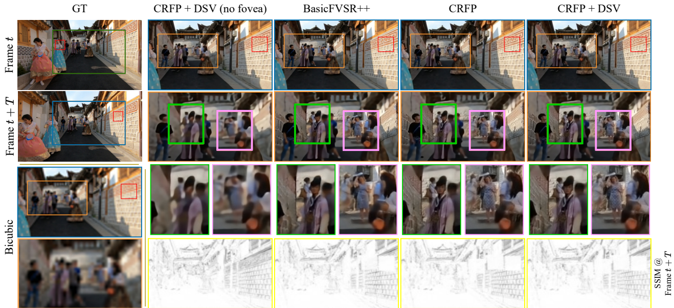
Figure 4. Visual comparison on the task of 8\times FVSR. The foveated region (red box) slides from left to right from frame t to frame t + T where T = 6 . PSNR and SSIM plots are for performance comparison, with brighter pixel value indicating higher performance.
