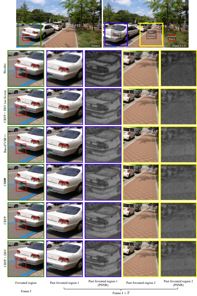
Figure 5. Comparison visual quality of past foveated regions across different methods. Two regions containing high frequency contents are shown. Refer to the license plate of the car and the tiles on the pavement to spot the distinction across different methods.
