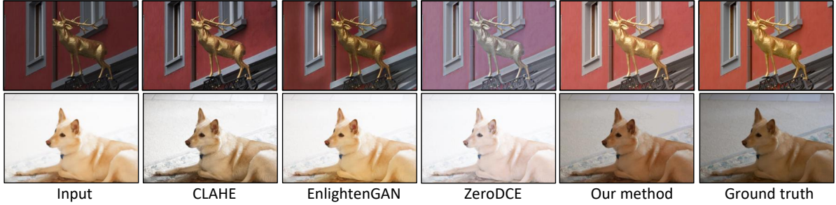
Figure 4. Visual comparison with unsupervised and traditional methods. In the under-exposure situation, CLAHE [28] and EnlightenGAN [10] could not brighten the image to a proper level, while ZeroDCE [8] tends to produce an image with washed-out colors. As for the over-exposed image, only CLAHE seems to produce an acceptable output whereas ZeroDCE and EnlightenGAN appear to fail to recover the image’s details in such a condition.
