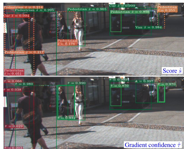
Figure 1. Object detection in a street scene. Top coloration: Score \hat{s} ; bottom coloration: instance-wise gradient-based confidence \hat{\tau} obtained by our method. Dashed boxes here indicate the discarding at any confidence threshold in [0.3, 0.85] . The top image contains FNs which are not separable from correctly discarded boxes based on the score (lower threshold would lead to FPs). In the bottom image, those \hat{s} -FNs are assigned higher confidences and there is a large range of thresholds with no FPs.
