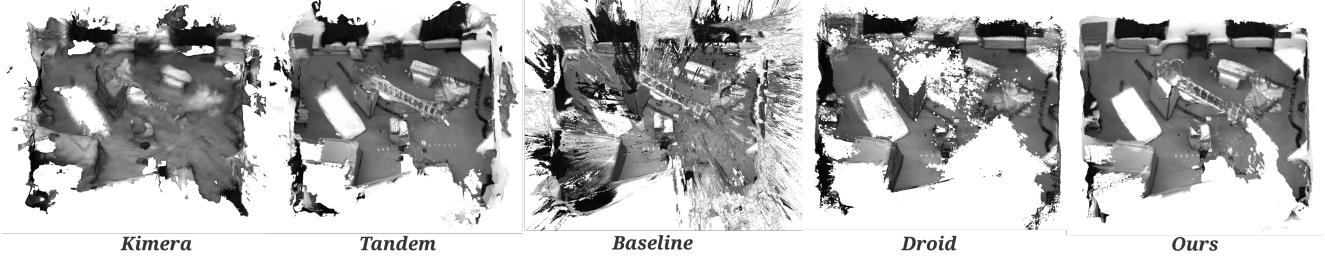
Figure 4. Comparison of the 3D mesh reconstructed by Kimera [17], Tandem [10], our baseline, and Droid’s depth filter [24] (using the default threshold of 0.005) versus our approach using a maximum tolerated mesh uncertainty of 0.1. EuRoC V2.01 dataset.
