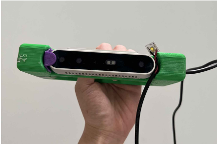
Figure 3. The simple set-up we used to record the datasets, an Intel Realsense D415 camera with an LED light attached to it.
