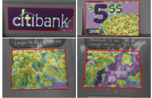
Figure 2. High weights of optic flow (yellow) appear mainly on corners and well-textured areas. Bottom: the POT-210 target with the highest average flow weights (left); weight values drop (purple) when "occluded" by a reflection (right). Best viewed in color.
