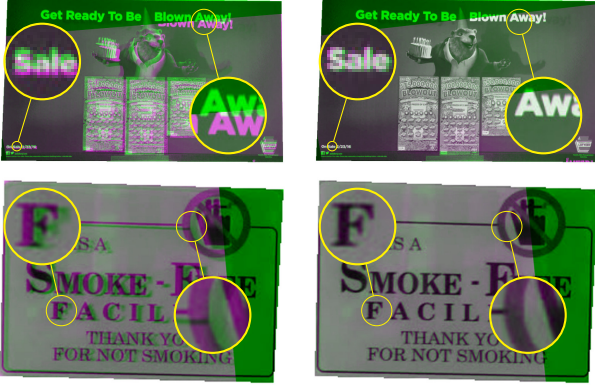
Figure 4. Precise re-annotation examples. Original ground truth annotation ( left ), improved ground truth annotation ( right ). The grayscale template in green channel, the GT-warped current frame in red and blue channels. Imprecise annotation causes green and magenta shadows, while precisely aligned images produce a grayscale result. The green bands on top and on right side respectively are caused by a partial occlusion on current frame. The alignment error of the original GT evaluated on the improved ground truth is 15.8px ( top ) and 7.2px ( bottom ).
