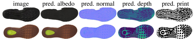
Figure 11: Failure cases. ShoeRinsics performs poorly in the presence of complex materials (e.g., translucence).
