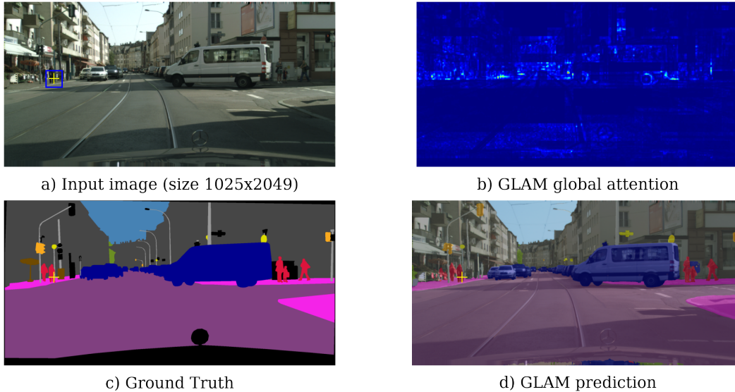
Figure 1. When segmenting the high-resolution image in a) with state-of-the-art multi-resolution transformers, e.g. Swin [24], the attention in the highest-resolution feature maps is limited to a small spatial region, i.e. the blue square for the yellow-crossed pedestrian. Our method incorporates GLocal Attention in Multi-resolution transformers (GLAM). The GLAM attention map for the pedestrian in a) is depicted in b): it captures both fine-grained spatial information and long-range interactions, enabling successful segmentation, as shown in d).
