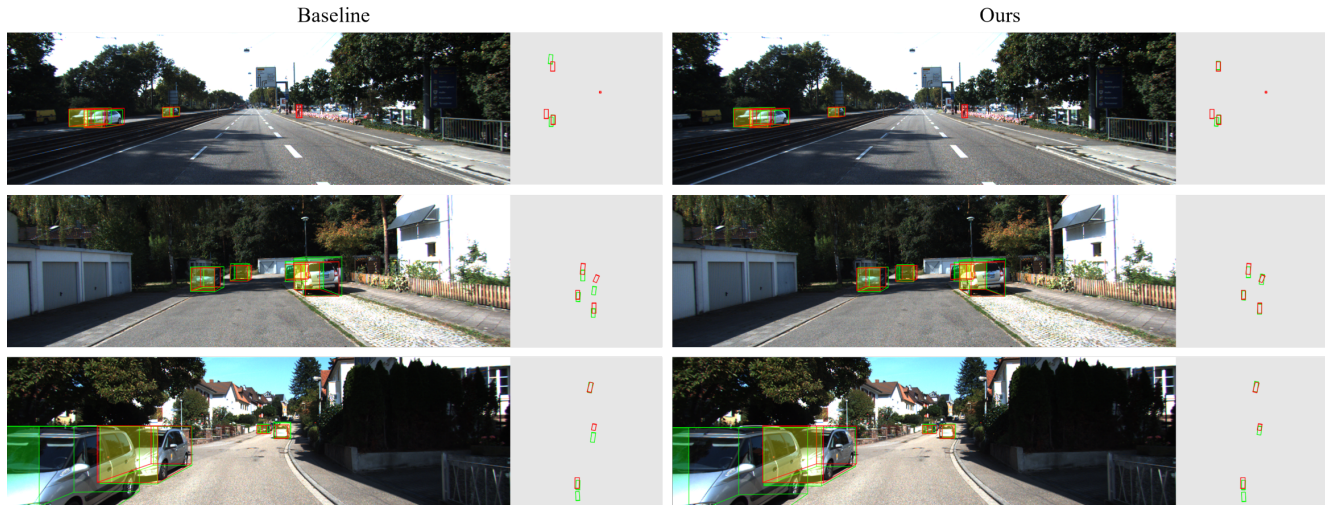
Figure 7. Qualitative results on the KITTI validation set. In each column, the image is on the left, and 3D detection results in bird’s-eye-view are shown on the right. The ground truths are in red, and the detections are in green. We achieve general improvements over the baseline.
