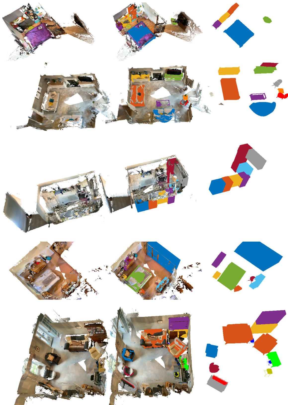
Figure 7. Results of our method for the ARKitScenes dataset. Left: RGB-D scan. Middle: Our results fused with the RGB-D Scan. Right: CAD model retrievals only.
