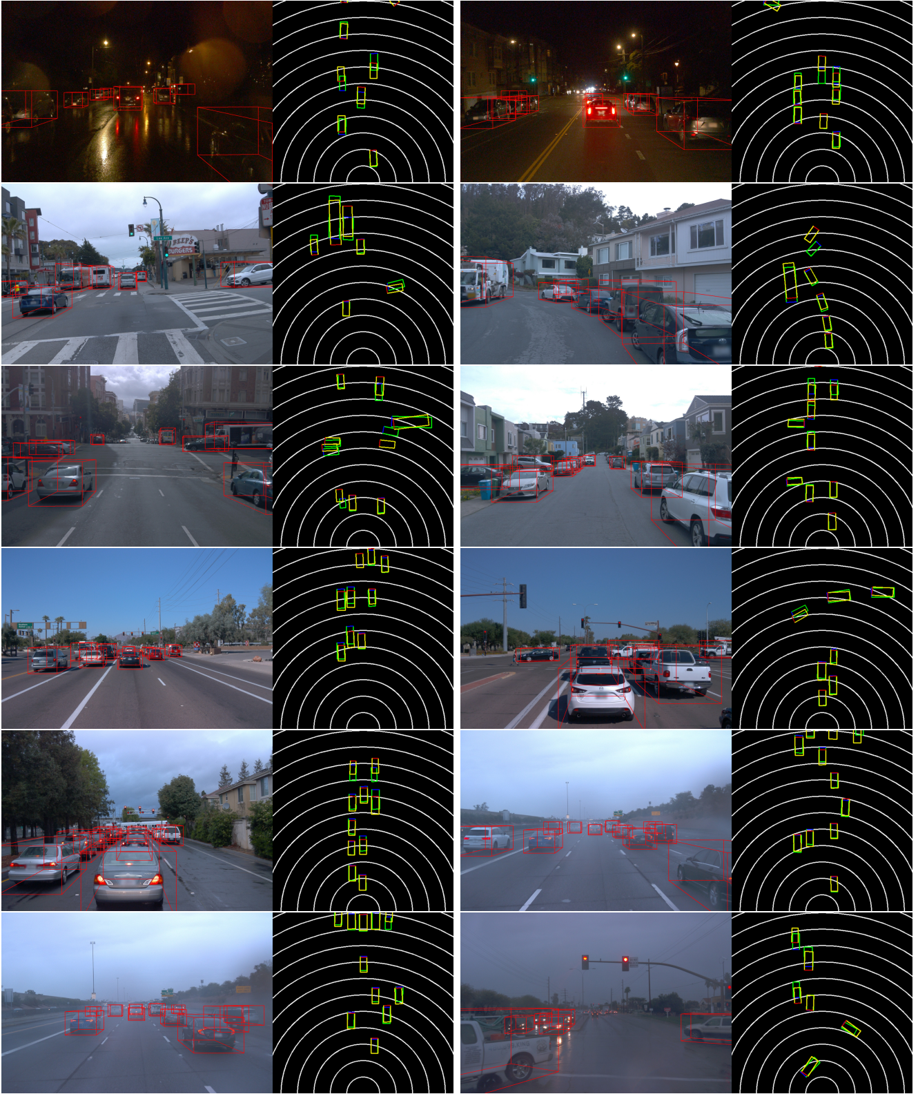
Figure 3: 3D detection results of MonoRCNN++ on the val set of the Waymo Open dataset [7]. MonoRCNN++ predicts accurate 3D bounding boxes for various challenging cases. The red boxes in the image planes represent the 2D projections of the predicted 3D bounding boxes. The yellow / green boxes in the bird's eye views represent the predictions and groundtruths, respectively, and the red / blue lines indicate the yaw angle. The radius difference between two adjacent white circles is 5 meters.
