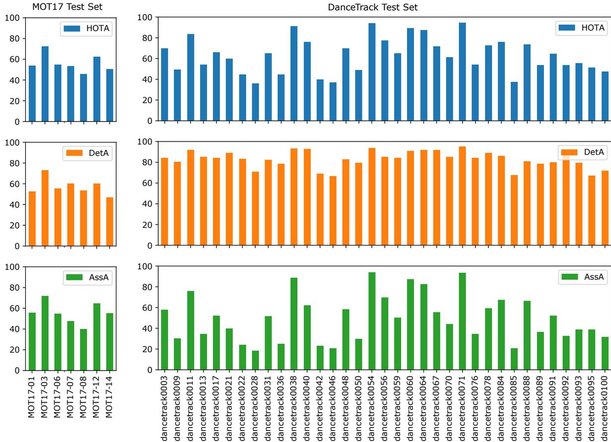
Figure 2: The tracking performance of each video on MOT17 test set [7] and DanceTrack test set [8]. On MOT17 test set, The data association performance (*i.e.*, AssA) is proportional to the detection performance (*i.e.*, DetA). On DanceTrack test set, for videos with the similar detection performance, the corresponding data association performance may have large differences, and therefore the data association performance may not be proportional to the detection performance.
