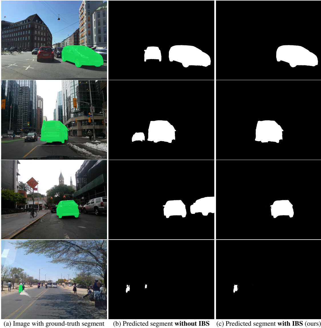
Figure 5: Confusion problem for crop-based training of Mask2Former for instance segmentation. Predictions for individual thing instances with and without IBS, on the Mapillary Vistas validation set. (b) The predictions by Mask2Former without IBS suffer from confusion, and (c) IBS largely solves this problem, leading to more accurate predictions. Full instance segmentation results for these images are shown in Figure 6.
