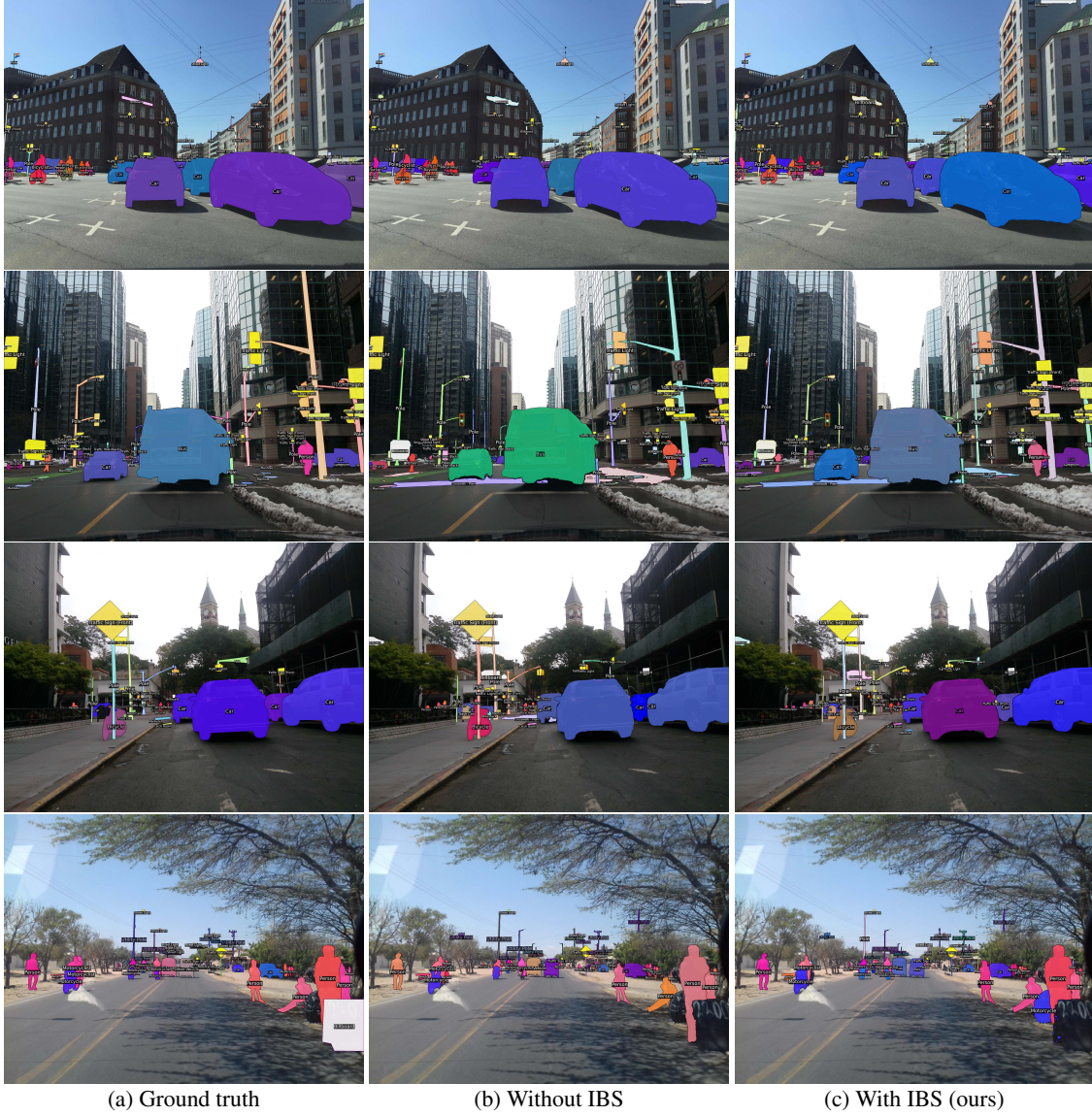
Figure 6: Intra-Batch Supervision on Mask2Former for instance segmentation. Images from the Mapillary Vistas validation set. Each instance is indicated with a unique color and text label, so confusion can be observed when multiple instances share a color or text label. Individual thing predictions for these images are shown in Figure 5. Best viewed digitally.
