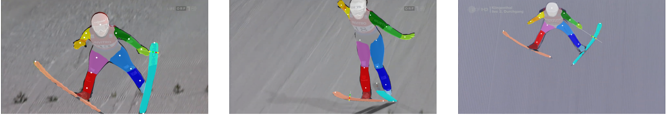
Figure 3: Examples for the ground truth keypoint generation process on skis. p is visualized in green, the orthogonal line in white, c_1 and c_2 in yellow and the generated point in red. The middle and right image show that the projection point can be located outside of a ski mask.
