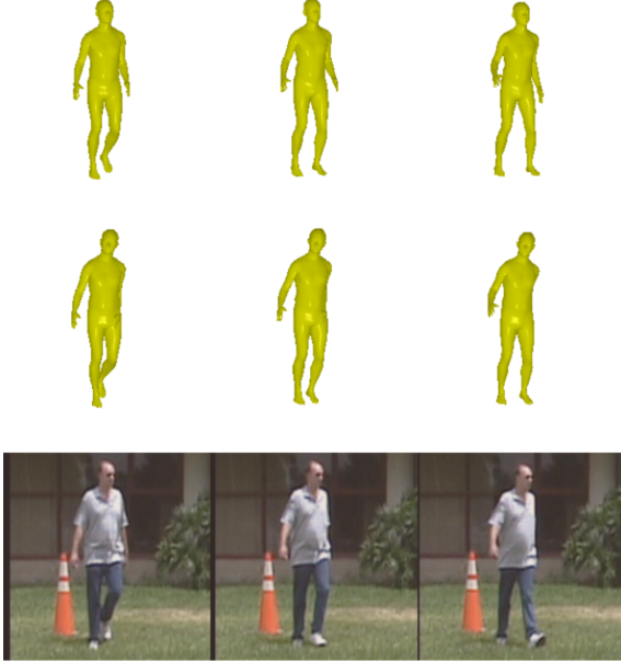
Figure 4. 3D body fitting results for a USF HumanID video (bottom) using VIBE (top) and GaitVIBE + Adv (center). Observe the improvements in the position of arms and legs obtained by GaitVIBE + Adv , which recovers the walking characteristics of the sequence. Meanwhile, the original VIBE output better approximates a standing position.
