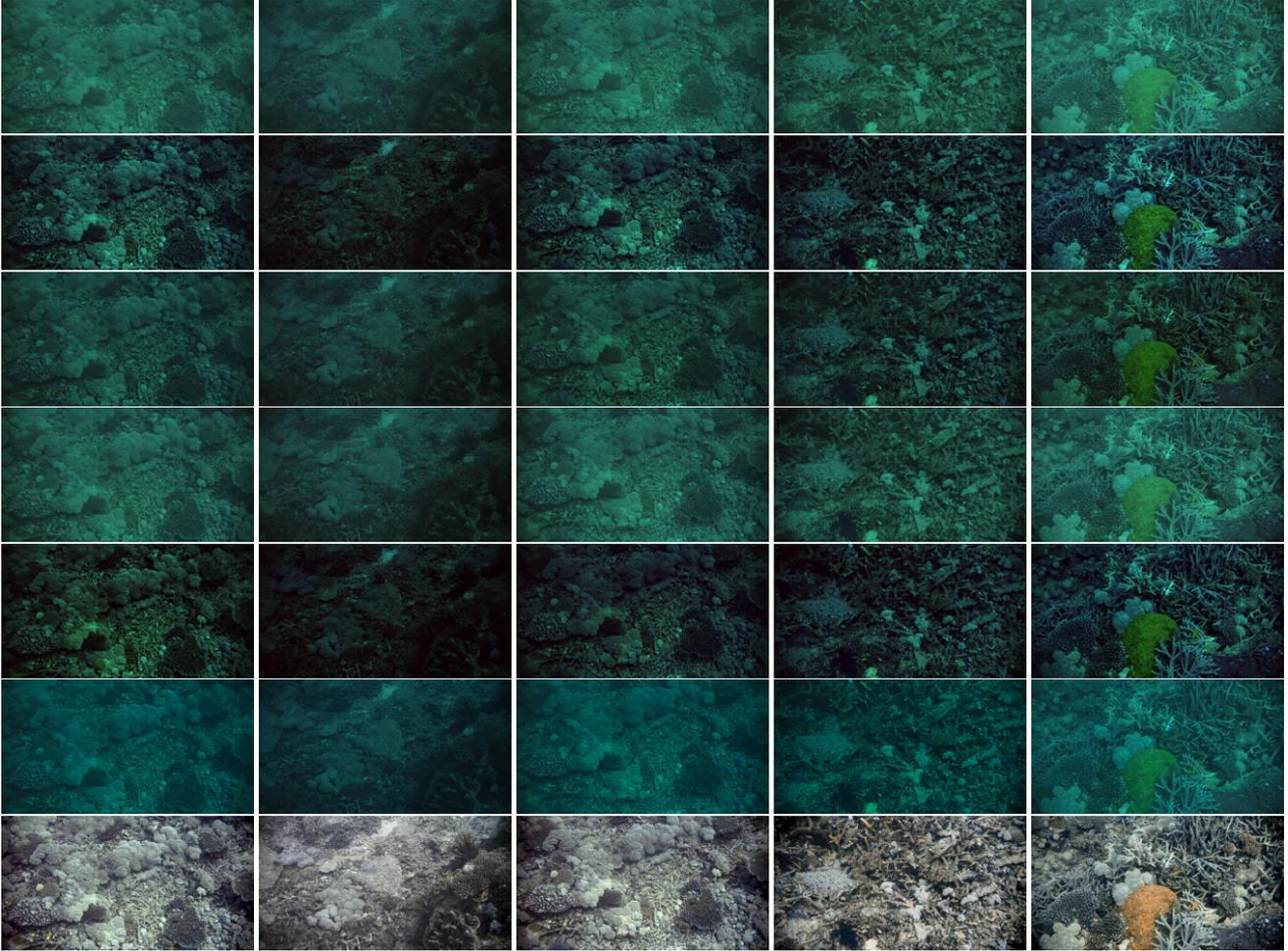
Figure 7: Restoration with non-learning based methods on HICRD dataset [17]. 1<sup>st</sup> row shows input images, 2<sup>nd</sup> row shows results from DCP method [19], 3<sup>rd</sup> row shows results from MIP method [5], 4<sup>th</sup> row shows results from RoWS method [6], 5<sup>th</sup> row shows results from UDCP method [13], 6<sup>th</sup> row shows results from ULAP method [36], last row shows results of the DepthCue (recovery of color and contrast is consistent throughout the scene).
