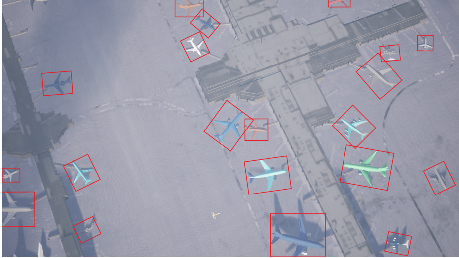
Figure 2: Example of the synthetic RarePlanes data. Real RarePlanes data shown in Figure 1
