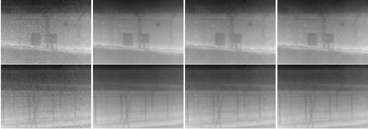
Figure 2. Online multi-view FPN removal on real microbolometer camera. Crops from 2 different views corresponding to averages (50 frames) to reduce temporal noise, and the corresponding results with our estimated FPN removed (adam) using 16 views (second row), bilateral-THPF (third row), SL-THPF (fourth row).
