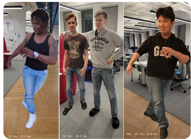
Figure 1. Three MoRF avatars (and a real person in gray) rendered on a mobile phone in real-time (at least 30 frames per second) in the augmented reality mode. Each of the avatars was created from a monocular video, while the poses and the camera positions of these examples differ from the training frames.
