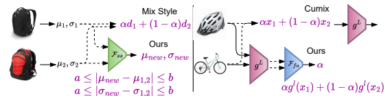
Figure 1. Differences between existing domain and sample interpolation methods (Mixstyle [55], Cumix [32]) and our proposed SODG-NET for style/sample synthesis. In both [55] and [32], \alpha is sampled from the dist. \mathcal{B}(\Gamma) , where we propose a learning based scheme. \mathcal{F}_{ss} and \mathcal{F}_{fa} denote the proposed style synthesis and feature aggregation blocks, respectively.
