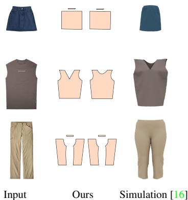
Figure 6. Qualitative results on real-world data. We reconstruct sewing patterns and perform drape simulation for real images.
