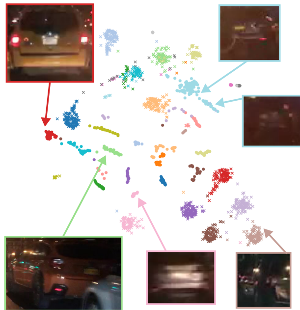
Figure 1. T-SNE projection of the predicted embeddings for the first 40 ground-truth objects in video b23f7012-fab06dac of the BDD100K validation set. Each color-symbol pair represents a ground-truth tracking ID assigned with DETR’s bipartite matching. Even during nighttime, the method can discriminate similar objects.
