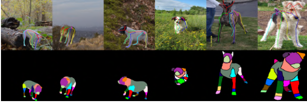
Figure 3. Examples from our Synth dataset (Columns 1–3) and PGT (Columns 4–6). (Top) Images with 2D keypoints overlaid. (Bottom) Part-segmentation maps. White-colored regions indicate unknown labels.
