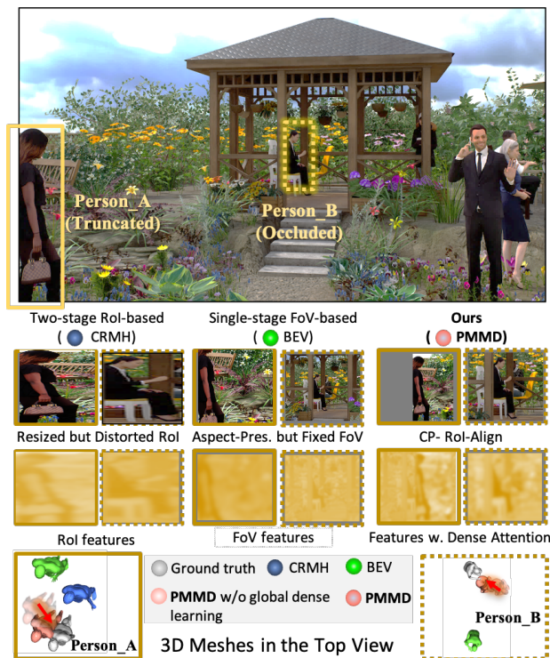
Figure 1. The proposed PMMD technical ideas, compared with CRMH [8] and BEV [28]. (Local Alignment) Center-Padding RoI-Align preserves the body aspect ratio and aligns body-to-RoI layout. (Global Dense Learning) Integrating local body-wise with global image-wise features to achieve precise translations.
