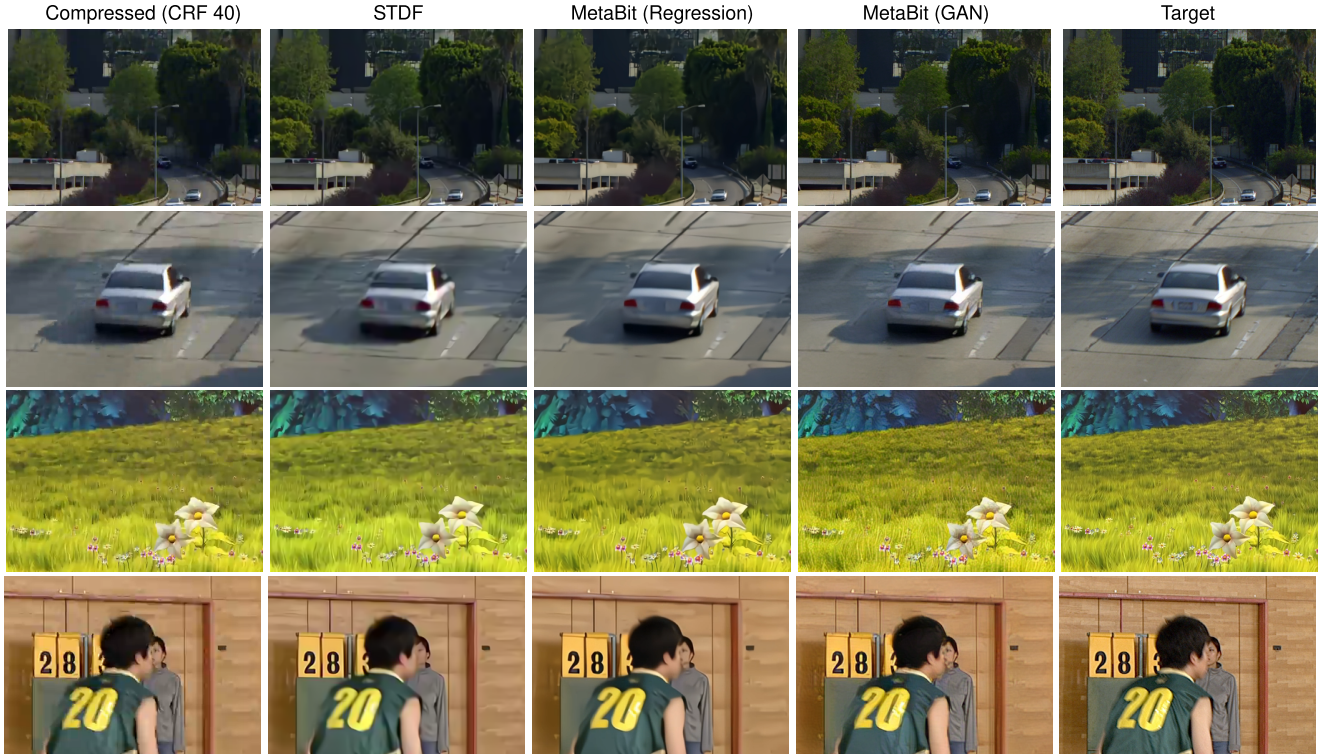
Figure 5. Qualitative Results. Please zoom in to view fine details. Note the increased quality of the MetaBit model over STDF and the enhanced sharpness and textures of the GAN method. This is particularly apparent on the trees (row 1), car (row 2), grass (row 3), and the wood texture (row 4). Additional qualitative results are shown in Appendix F and the attached supplement.
