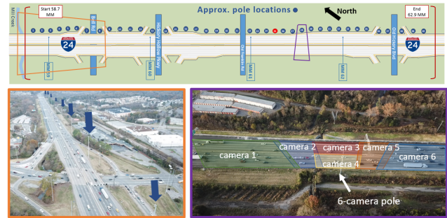
Figure 2. (top) Graphical overview of the I-24 MOTION system. Each blue dot represents a camera pole with 6 cameras. Red dot indicates a camera pole outage (Pole 25). (orange) drone image showing 8 of the 40 system camera poles. (purple) Typical 6 camera per pole coverage layout. Best viewed zoomed-in.
