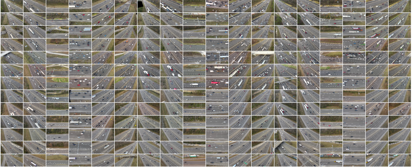
Figure 1. Example fields of view from each of the 234 cameras included in the I24V dataset. Each camera is recorded in 1920 \times 1080 resolution and at 30 frames per second. Scene information is provided for each roadway direction of travel in each camera.
