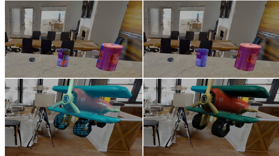
Figure 6. Selected examples of the benefits and drawbacks of using the final mask-refinement step with SAM. Left: Mask predictions using no SAM refinement. Right: Mask predictions with SAM refinement. Notice that SAM refinement helps with multiple object instances of the same class, but decreases the performance when the object consists of multiple parts.
