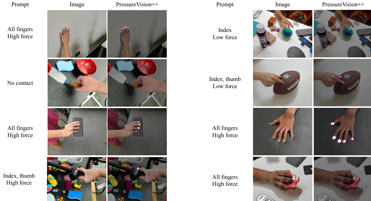
Figure 6. Results on the surfaces in the weakly labeled test set, none of which are included in the fully labeled training set. PressureVision++ produces qualitatively accurate results on highly textured, curved, and compliant surfaces. All images except the top row are zoomed in to show detail. The bottom right shows a failure case where pressure is underestimated on an object.
