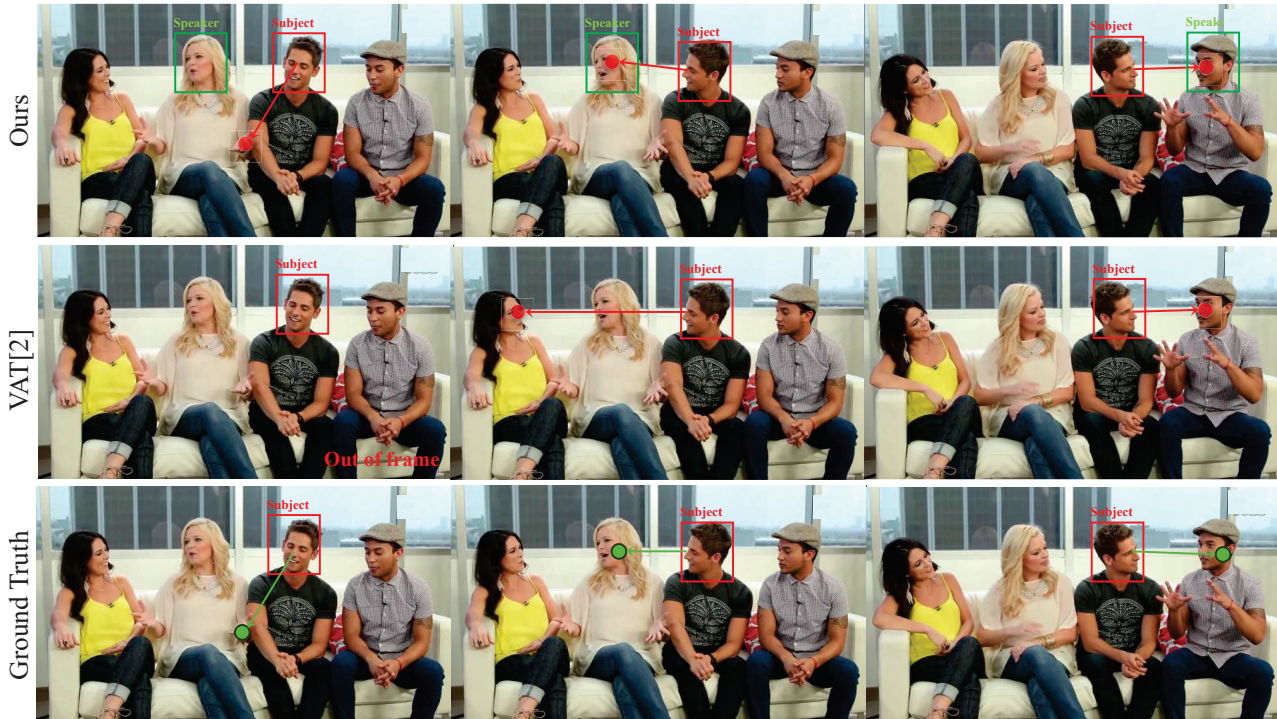
Figure 4. Comparison from Gaze Candidate Estimation model and VAT model. The first line is the output of gaze candidate estimation model, the second line is the output of VAT model, and the third line is the ground truth. Our model outperforms the VAT method in accurately detecting the gaze target. In the first frame, our model accurately detects the gaze target where the VAT method failed to do so. This demonstrates the superior performance of our model in terms of gaze target detection. In the second frame, our model accurately detected the speaker as the gaze target in a conversational scenario, while another model failed. Incorporating audio cues is crucial for gaze following, and audio-visual fusion can significantly improve accuracy, especially in real-world scenarios.
