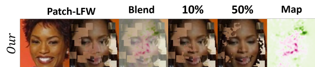
Figure 1. An example visualization of our proposed efficient explainable face verification explanation, xSSAB, on the novel Patch-LFW benchmark and its evaluation protocol. The added patches from an imposter identity on an original genuine pair shifted the model’s decision to non-match. During the evaluation, the added imposter clues (patches) are replaced by the original pixels based on the identified dissimilar area (pink) of our approach.
