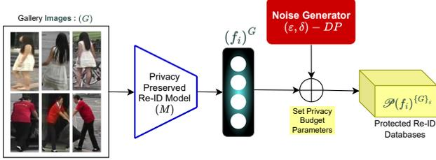
Figure 4. Illustration of controllable privacy with differential privacy. Features  $(f_i)^G$  are extracted from a trained Re-ID model  $\mathcal{M}$  for gallery  $\mathcal{G}$ . The image perturbation generates Gaussian noises with a given  $(\epsilon, \delta - DP)$  for  $(f_i)^G$  to generate a protected gallery  $\mathcal{P}(f_i)^{G, \epsilon}$ . A query  $q_i$  can then be used to retrieve the closest matching results from  $\mathcal{P}(f_i)^{G, \epsilon}$ .
